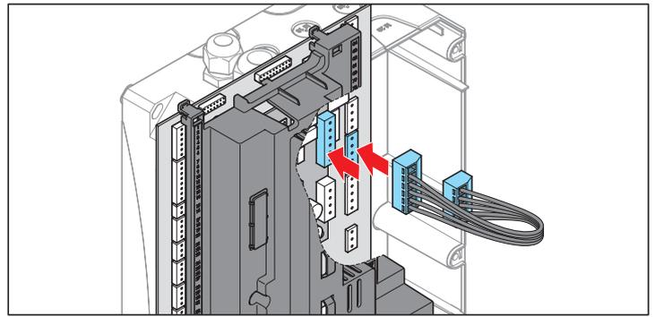
6. Connect the control unit and the induction loop module with the connecting cable.
