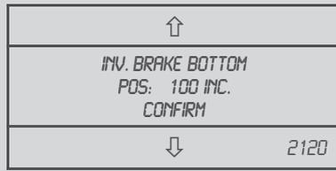
Switchpoint of brake (brake point) for end position bottom (ELu), as difference from ELu.
