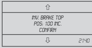
Switchpoint of brake (brake point) for end position top (ELu), as difference from ELu.
