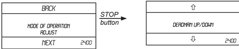
Select mode of operation with the  $\uparrow$  and  $\downarrow$  buttons and confirm with the STOP button.
